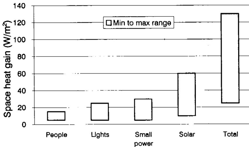
Figure 2 Typical range of space heat gains in office buildings
