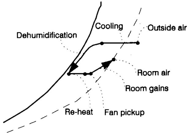
**Figure 12 Cooling and dehumidification on a psychrometric chart**
