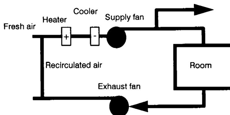
*Figure 8 Simplified schematic*
