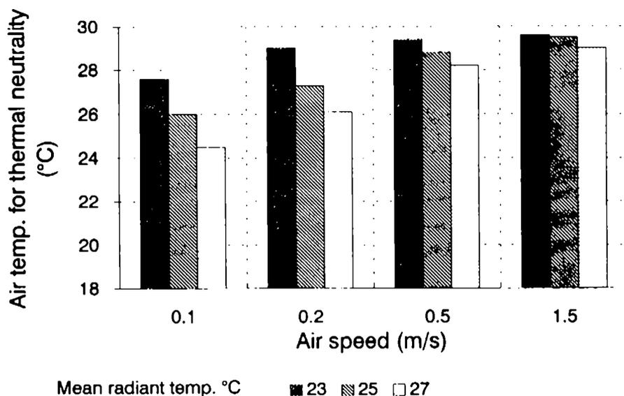
Figure 3 Effect of air speed and mean radiant temperature of the enclosure on thermal comfort
