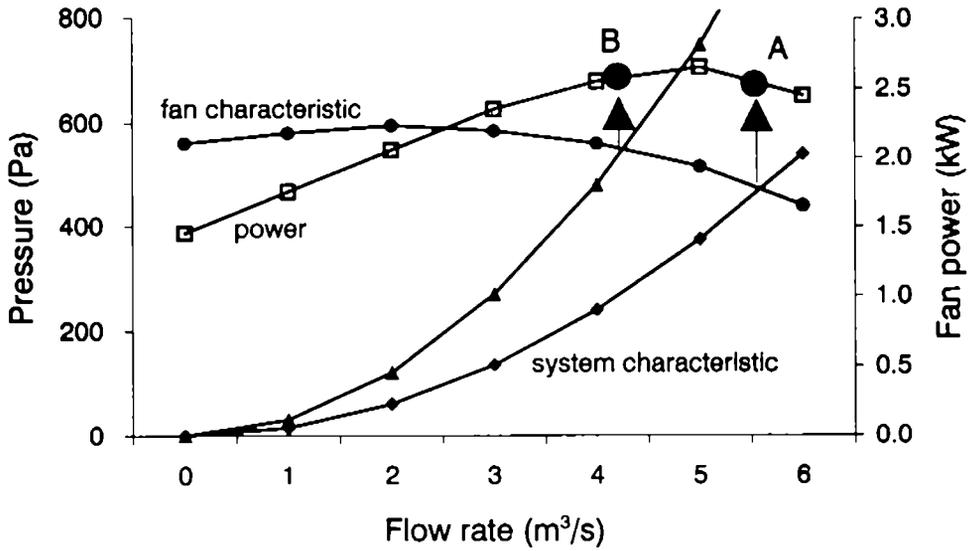
Figure 17 Controlling flow with a damper
