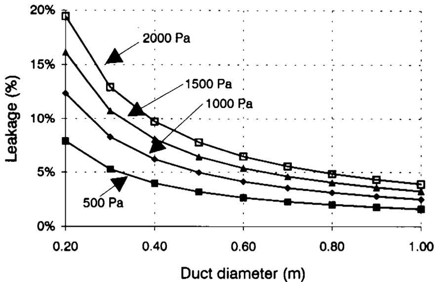
Figure 15 Effect of pressure and size on leakage
