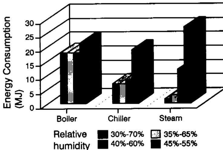
**Figure 13 Effect of humidity control on energy consumption**
