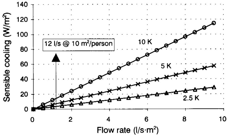
Figure 1 Ventilation for cooling and IAQ
