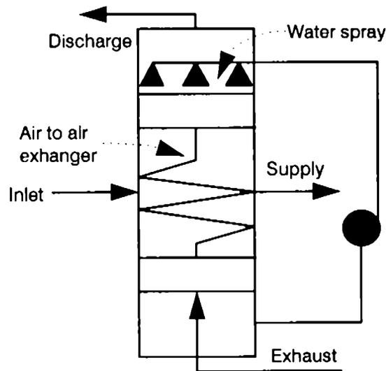
*Figure 6 Indirect evaporative cooler*
