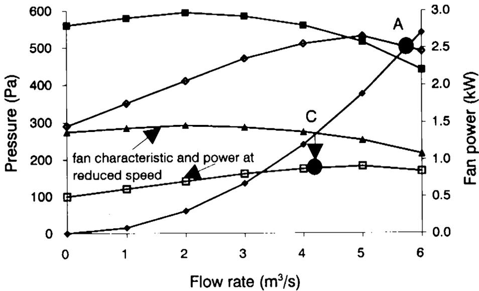
Figure 16 Controlling flow with speed control
