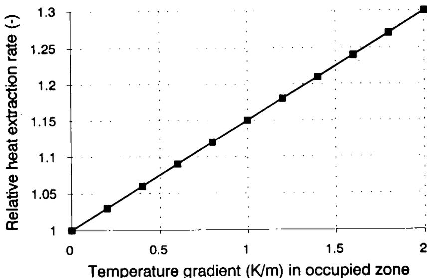
Figure 10 Effect of temperature gradient on heat extraction rate
