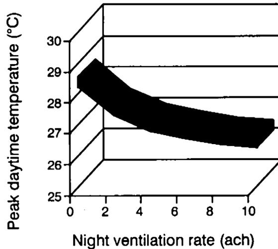
*Figure 11 Effect of night ventilation on peak daytime temperature*
