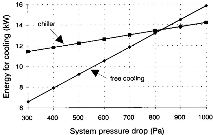
*Figure 18 Comparison of free cooling and chiller cooling*
