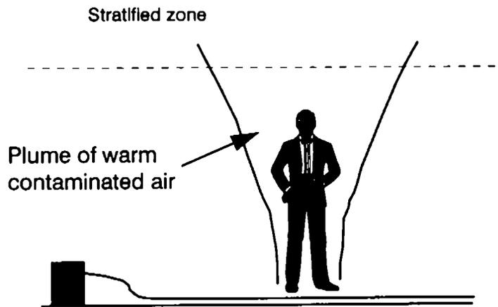
Figure 9 A displacement ventilation system
